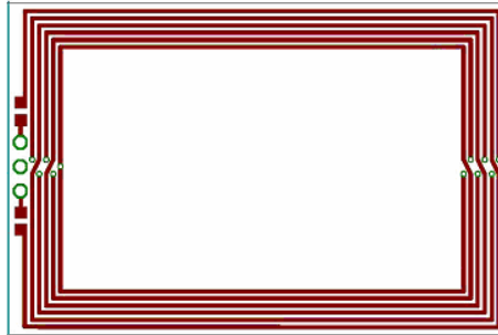
Fig 28. PN511/PN531 evaluation board antenna
