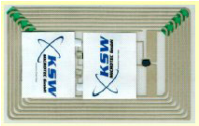
Figure 1 The TempSense active label which is the size of a credit card but thinner
