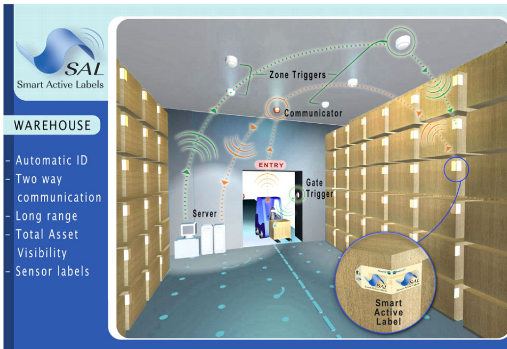
Fig. 1.6 SAL-C concept of a warehouse managed using disposable SALs on packages. These would be in semi- active mode to achieve range without being too demanding of the thin laminar batteries.
