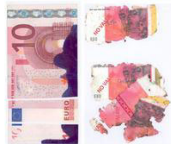
Ink staining versus acid.
