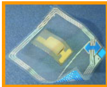
Fig. 4.10 Infinite Power Solution flexible lithium battery as part of a semi-passive tag.
