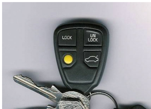
Fig. 1.7 An active RFID car clicker working in semi-active mode at 433 MHz
