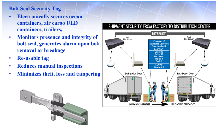
Fig. 1.14 Sealing and anti-tamper capability with intermodal containers
