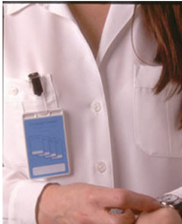
Fig. 5.3 Identec semi-active RFID personnel tag. It has three meters range and is dormant when out of range. Safety is a major benefit.
