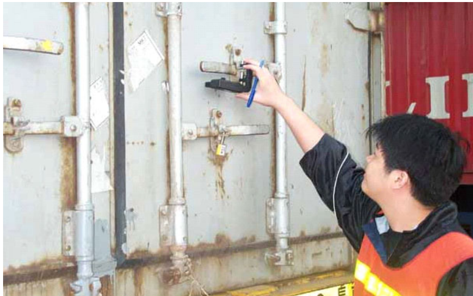
Fig. 1.15 Smart and Secure Tradelanes active RFID seal being used to lock an intermodal container
