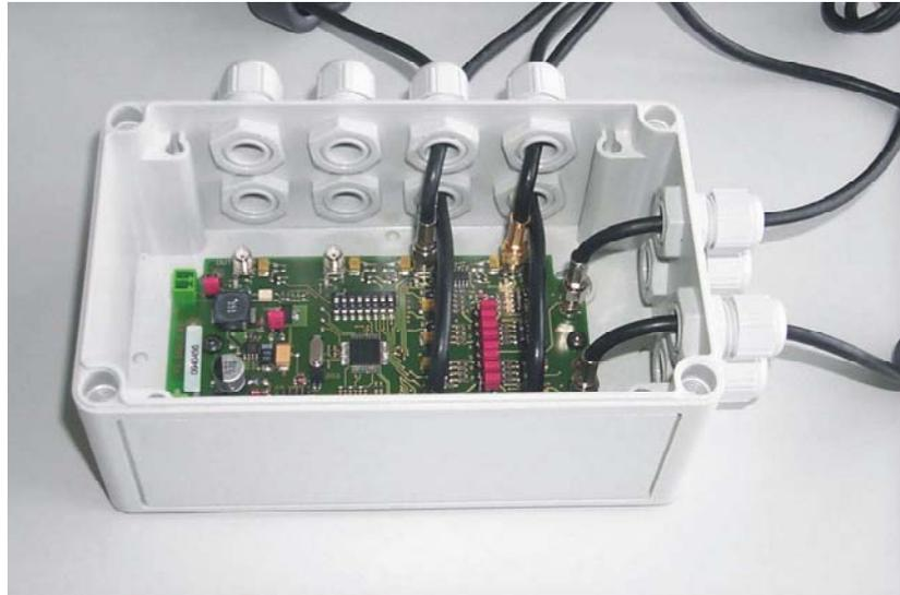
8 times Multiplexer for OBID i-scan<sup>®</sup> readers\* with external antenna connection for operation of several single- or gate antennas with only one reader.
